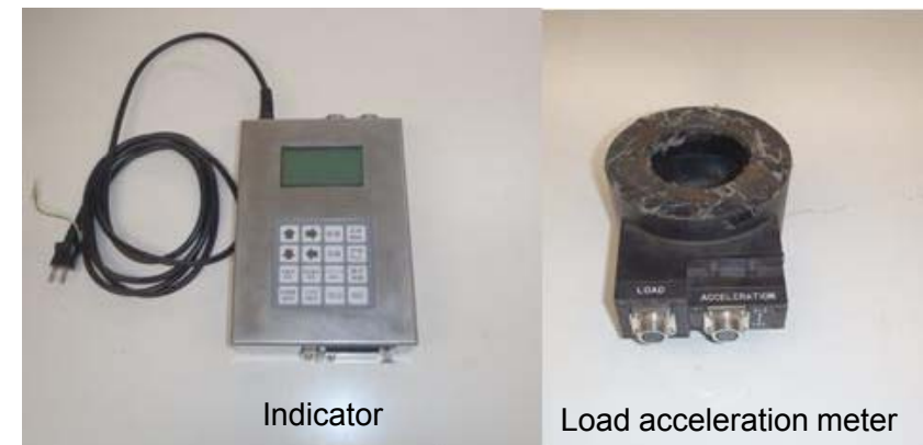
Rapid loading test device incorporated into the pile driver
