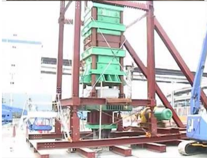
56t plumb bob, maximum drop height: 3 m
